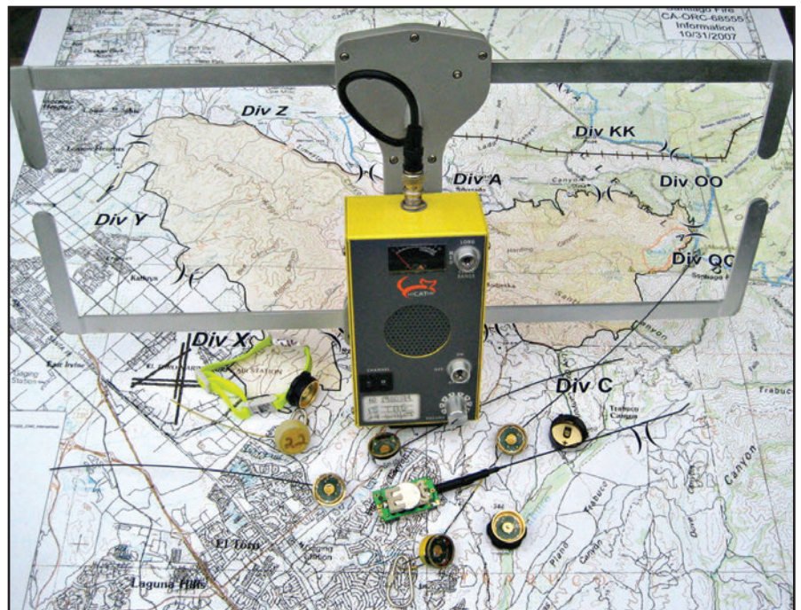
Photo F. A Moxon direction-finding antenna is part of Communications Specialists' flea-power, 222-MHz radio system. The antenna folds up nicely when going portable.
