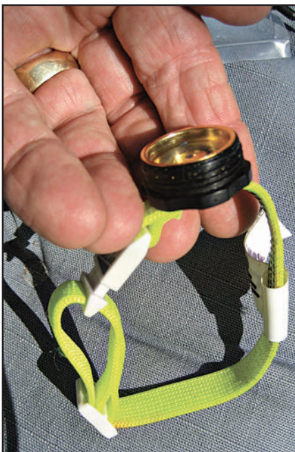
Photo E. This small ticker-tag is a 222-MHz, 1-milliwatt, 20-millisecond tag collar that has a variety of uses for the communications hobbyist. Put one on Fido, and you're likely never to have a lost dog again. Visit Communications Specialists' website at < http://www.Comm-Spec.com >.
