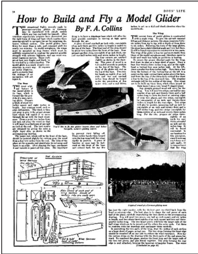
Photo D. The September 1931 edition of Boys' Life magazine was the inspiration for what would become the Radio Boys' Hammarlund Flyer Antenna. F.A. Collins based his 46-inch wingspan model glider on what was called "the flying wing." (Courtesy of Herbert Wallace)
