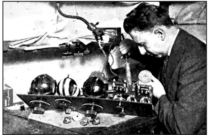
Photo C. “A boy built this outfit for $27.80. It is a three-circuit regenerative detector with detector and two-stage amplifier and would cost between $100 and $130 if purchased ready-made.”
