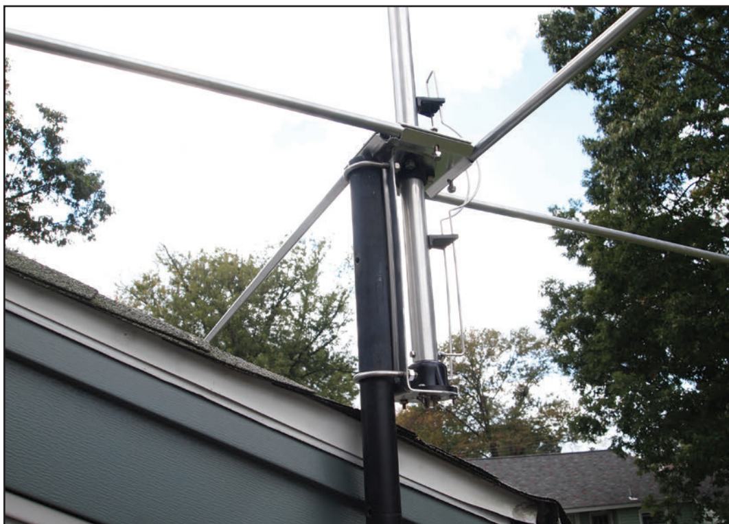
Photo A. Here's a close-up of the mounting hardware for the Hy-Gain SPT-500 Super-Penetrator vertical at WPC2CS in Southern New Jersey. The base of the antenna was mounted significantly below the peak of his home's roof to comply with FCC CB antenna height rules. (Courtesy of WPC2CS)
