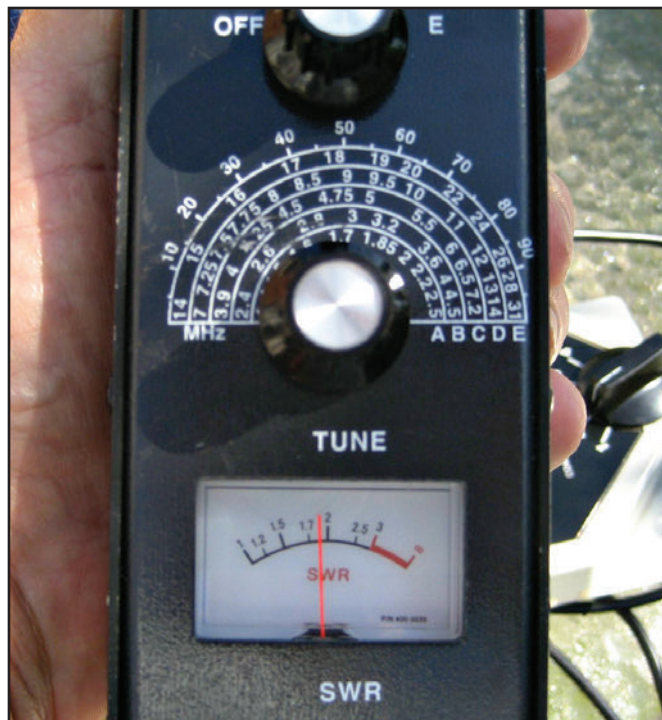
Photo B. With the MFJ-207, “simply run the coax into the analyzer and sweep the tuning knob near the frequencies the antenna is designed for,” writes WPC6NOA. “When the SWR meter dives back to the start pin, you know the antenna is tuned.”
