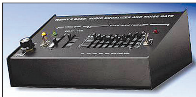
Photo C. Even if your rig has an internal EQ, W2IHY's 8-Band Audio Equalizer and Noise Gate is pretty much the gold standard when it comes to amateur radio audio processing. The EQ provides many additional functions, which you can explore at http://www.w2ihy.com . See the stellar reviews for this unit at http://bit.ly/1fHRsFN . (Courtesy of KPC0ZZZ)
