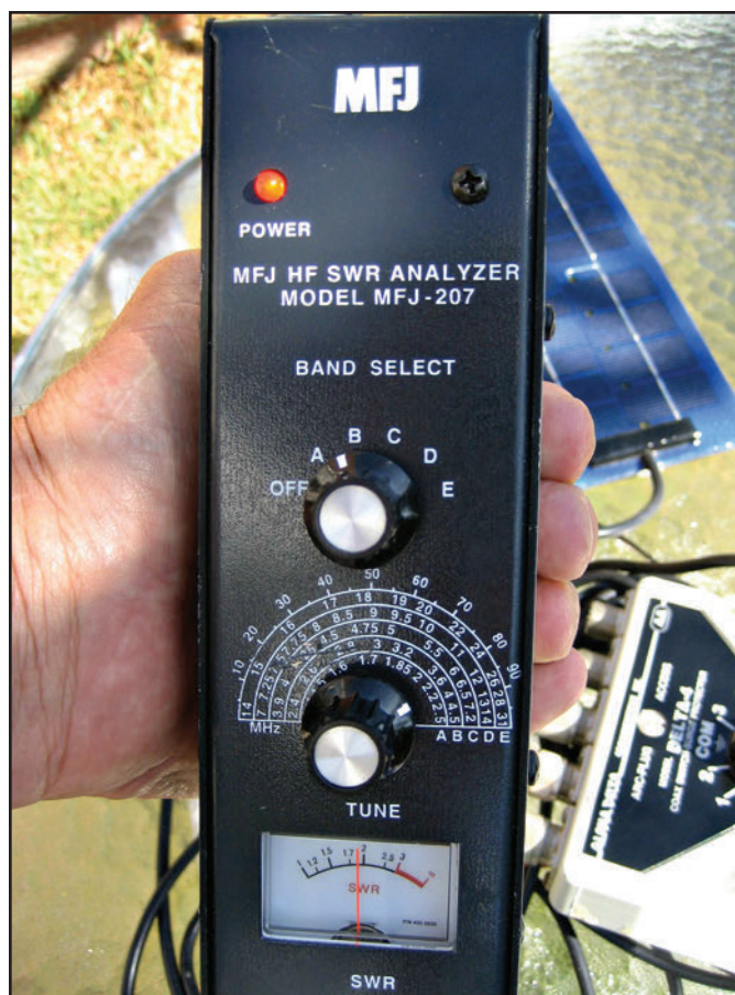
Photo A. An oldie but definitely a goodie, the MFJ Enterprises MFJ-207 Antenna Analyzer is an excellent and affordable test instrument that won't break your bank. Check it out at < http://bit.ly/16zYlkt >. (Photography courtesy of WPC6NOA)
