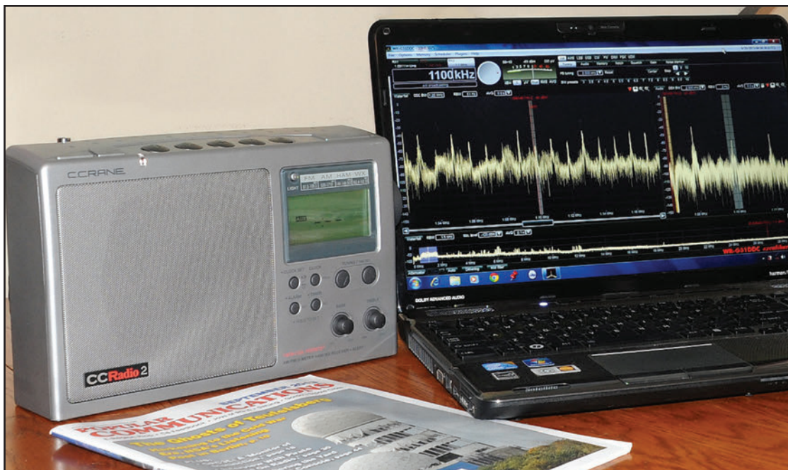
Photo A. The CCRadio-2 is not only an excellent portable AM receiver, it serves as an amplified external speaker for a laptop SDR. (Courtesy of WPC1CAT)
