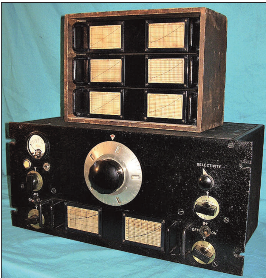
Photo G. National HRO superhet receivers covering 1.7 to 30 MHz with four plug-in coils, were issued to Britain’s VIs to intercept enemy signals from 1941 to 1945. They were imported from the United States under a Lend-Lease agreement set up by President Roosevelt. After the War, VIs were allowed to buy the receivers at a reduced price. (Internet screen grab from RadioBlvd.com < http://bit.ly/1fuT8oy >)
