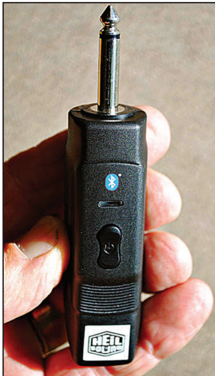
Photo G. The Heil Wireless PA System features a Bluetooth™ receiver that plugs into the 0.25-inch phone jack on any PA system or audio equalizer.
